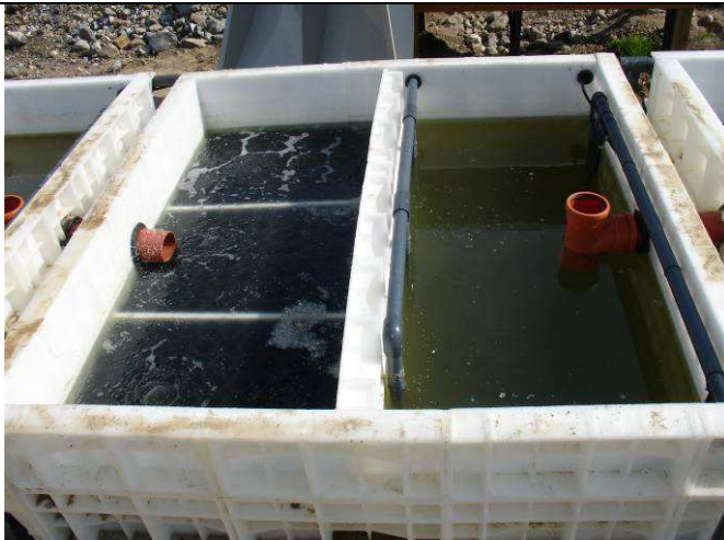
3 step Jupiter 25 system. To achieve the required cleaning, a 3 chamber Jupiter system is required.
